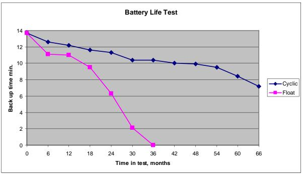
Figure 3: Long Term Cyclic Charge vs. Float Test
