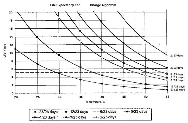
Figure 4: Calculated Service Life Extension for ABM Charge Algorithm
