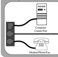
The included cable and software (Back-UPS ES 525 only) provide automatic file saving and shutdown of the operating system in the event of a sustained power outage
